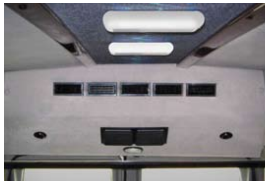
Our standard 28,500 BTU rear AC and floor heat systems, combined with 3 1/2" of extreme weather sidewall and ceiling insulation, provides passengers maximum comfort in all climates.
